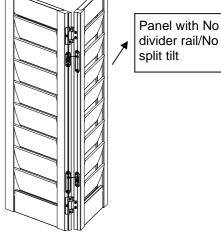
When there is more than one louver sections (with divider rail/ split tilt)
