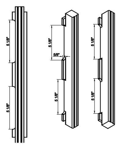
d. **C cutout**---Crank cut outs (C1 cutout, C2 cutout, C3 cutout): (Always on bottom of bottom frame. Available in all styles of the L-frames and all sill plates.)
