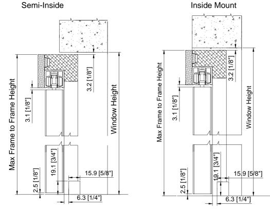
For frame hinged bifold track shutter used as door, the bottom gap will be 3/4" by default. Please specify "Used As Door" on the order form.
