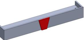
The keystone will be installed by screws. We will pre-drill the screw holes and the screws will be packed in hardware box.
