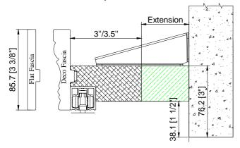
For 180 Bi-fold, if Bottom Pivot L Bracket is required, the extension for the L shape light block will be 1 3/4" in width. Please see picture below:
