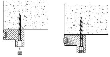
90 Degree Bifold Track & Floating Panels Hanger Location:
