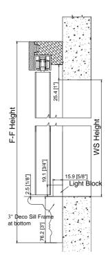
Note: For OM Frame Hinged Bifold shutter not to use as a door, if there is no existing sill at the bottom of the window opening, it is recommended to have the 3" Deco Sill Frame at the bottom.
