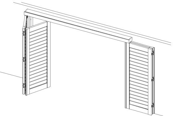
• Track is pre-installed on the header; standard 1 track only.
