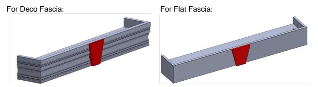
The keystone will be installed by screws. We will pre-drill the screw holes and the screws will be packed in hardware box.
