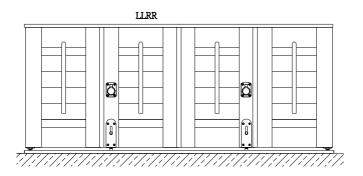
The Panel Lock location for both track system shutters and regular shutters would be the same.
