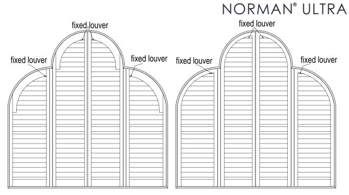
Horizontal louvers center arch with quarter round side panels -Standard louvered arch Horizontal louvers center arch with quarter round side panels -Continuous arch
