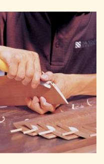
The secret to a handsome and durable shutter finish really isn't a secret at all. It takes multiple sequences of sanding with progressively finer sandpaper to open the pores of the wood for coating and smoothing the surfaces. Each layer is finely coated with high-quality stain or solid color. This labor-intensive process is the only way to achieve the translucent, deep finish of a Sussex Shutter.
