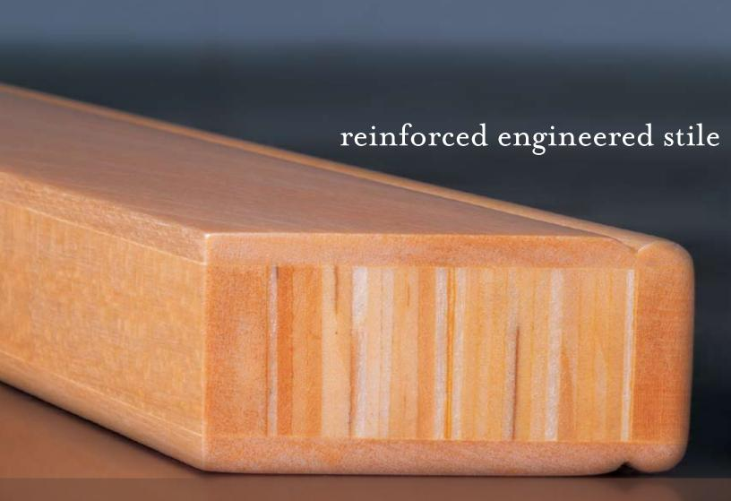
TO INHIBIT WOOD DEFORMATION, BONDING MULTIPLE LAYERS OF WOOD TOGETHER WITH PRESSURE, HEAT, AND A PROPRIETARY FORMULATION CREATES THE CORE OF NORMAN'S REINFORCED ENGINEERED STILE.
