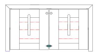
4. Note: if panels only with side magnets and there is no standard magnet on the back of panels, panels may open for external factors.
