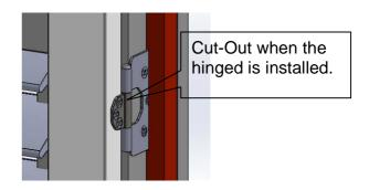
4. Direct Mount 3" Hinge is not suitable for drywall installations.
