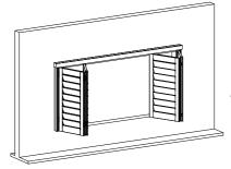
Note: For OM Frame Hinged Bifold shutter not to use as a door, if there is no existing sill at the bottom of the window opening, it is recommended to have the 3" Deco Sill Frame at the bottom.
