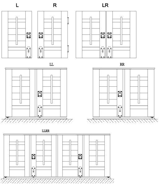
The Panel Lock location for both track system shutters and regular shutters would be the same. The general principle is that the Panel Lock position will avoid the stile which will install the spring-loaded guide at bottom (same stile as the Wheel carrier).
