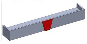
The keystone will be installed by screws. We will pre-drill the screw holes and the screws will be packed in hardware box.
