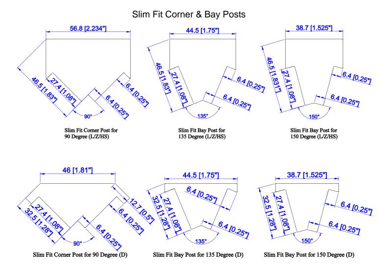
Note: Due to size and weight limitations, Slim Fit Posts may only be hinged on one side and with a single panel (no bi-folded panels). Please consider this when determining panel configuration.
