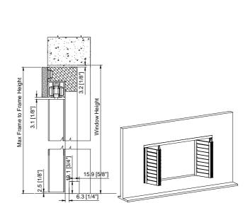
For frame hinged bifold track shutter used as door, the bottom gap will be 19mm by default. Please specify "Used As Door" on the order form.
