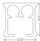
CCS® CONTRACT CORD SYSTEM Aluminum extrusion, white, powder coated, lubricated. Available in 25 white, 65 brown and 90 silver. All corded systems include child safety tension device.
