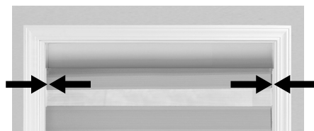
Inside Mount Light Gap Refer to Light Gap Chart
