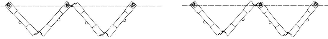
**180 Degree Bifold Track Panel Hanger Location:**
