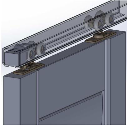
Push wheel carrier into the wheel carrier bracket to seat
