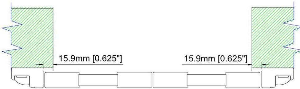
Side view for module in panel with different louver types
