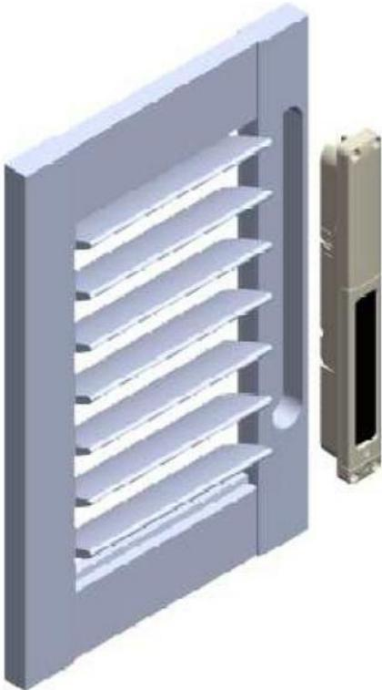
Module Location: (Invisible Tilt will be on the same side as the module)
