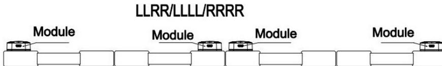
Given the need for module clearance, the following OM install frames will require either a build out or extension of at least 1/2" (12.7mm) when the modules must be located on the outermost stiles as outlined above:
