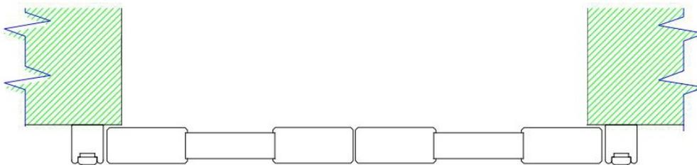
L Frames with a light block thickness less than 3/4" (19mm) flush with the window opening
