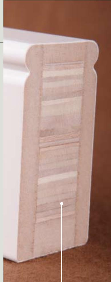
TO INHIBIT DEFORMATION, BONDING MULTIPLE LAYERS OF WOOD TOGETHER WITH PRESSURE, HEAT, AND A PROPRIETARY CHEMICAL FORMULATION CREATES THE CORE OF NORMAN SHUTTERS REINFORCED ENGINEERED STILE.
