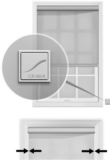
Inside Mount Light Gap Refer to Light Gap Chart
